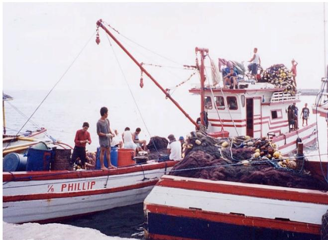
Figure 3. Purse-seiners in Tambler with power blocks and large fishing nets onboard (DOTC-PMO, 2003)
