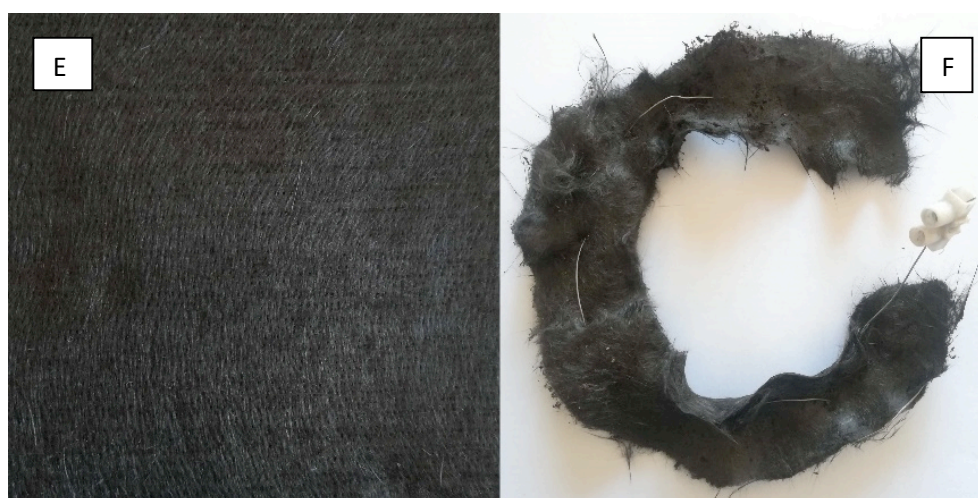
Figure 4 : CARBISO™ M 100% Recycled Nonwoven Mat. C) detail of the recycled nonwoven mat; D) the cathode used in recycled carbon felt configuration
