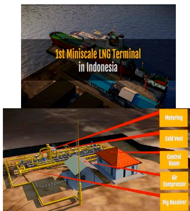
Figure 3. Illustration on Mini-Scale LNG Facility that has been built and initiated by PT Indonesia Power UP Bali, introduced as energy efficiency innovative effort for Pesanggaran Power Generation.
