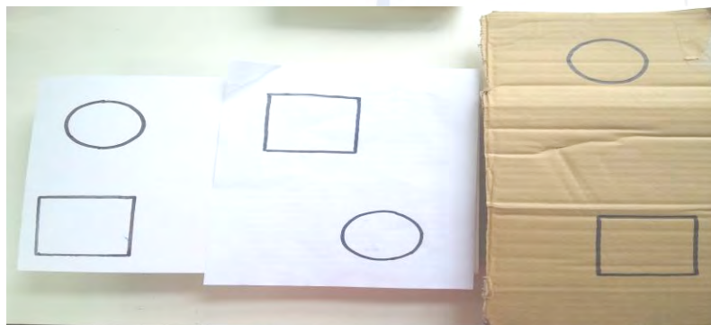
Figure 2 The circle (radius 50 mm) and square (100 x100 mm) for cutting path have been drawn on three types papers.
