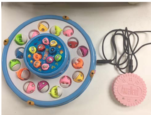
Fig. 5 A modified Toy and a Special Switch Connected with an Audio Cable
