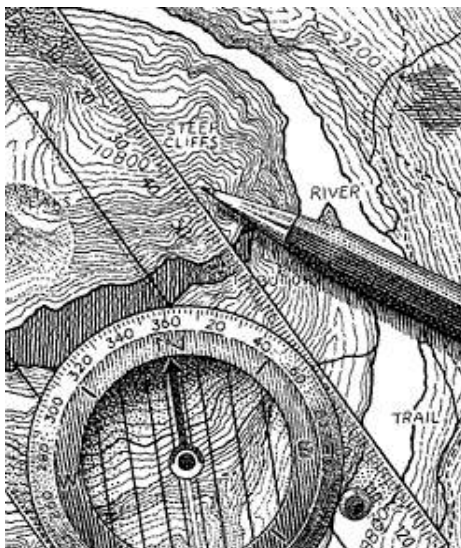
Fig 13. Contour lines in map are drawn to describe imaginary lines that cut across the form.
