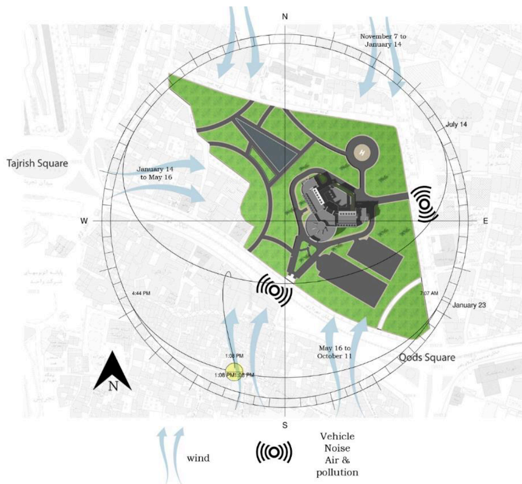
Figure 2. The site analysis shows the different wind directions, different sun altitudes between summer and winter, and the directions of the most noise and polluted streets.
