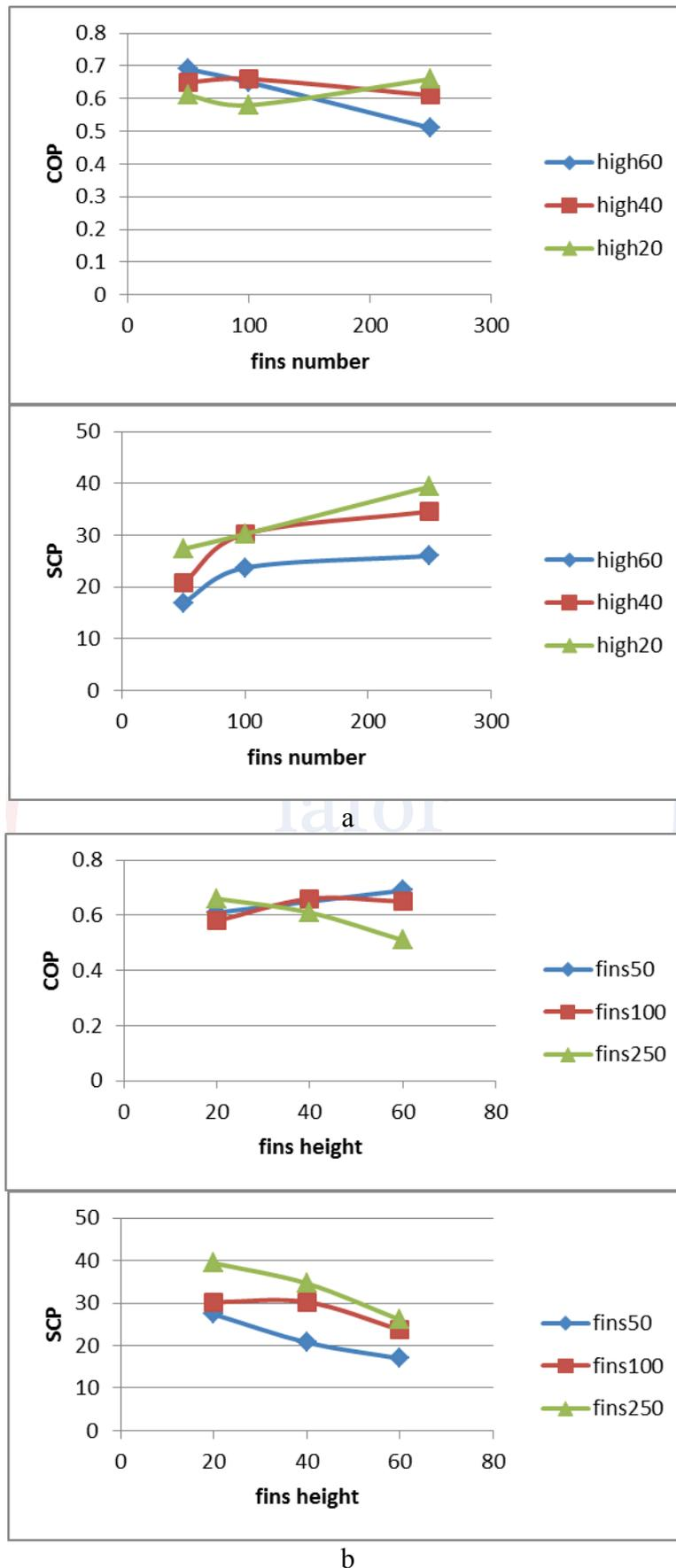
Fig.5 (a) variations of the COP and SCP with fins numbers with different fins height. (b) Variations of the COP and SCP with fins height with different fins numbers.
