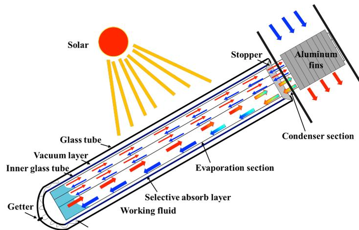
Figure 4: Working principle of the collecting unit.
