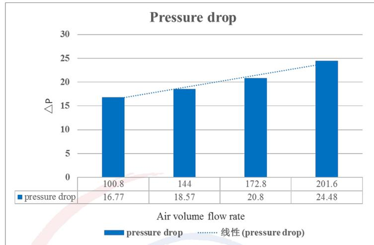
Fig. 11: Pressure drop of the EVSAC with MHPA.
