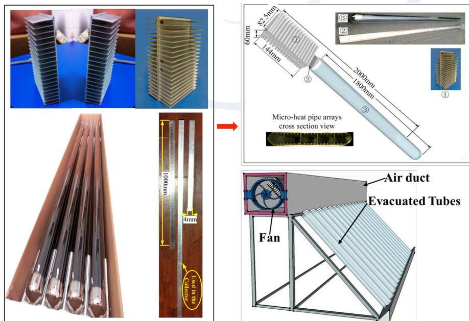
Figure 3: Structure of ETSAC with micro-heat pipes arrays (MHPA).
