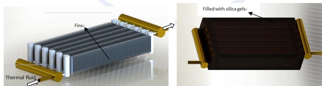
Fig.1 adsorbent bed
