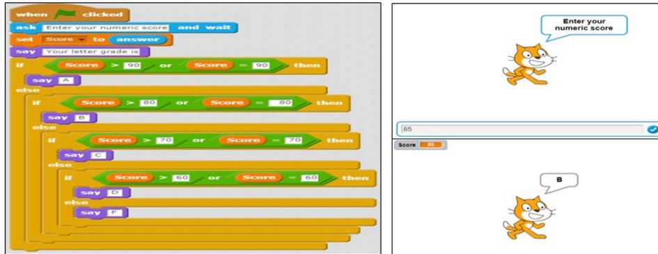
Figure 3. Scratch block-coding for letter grade
