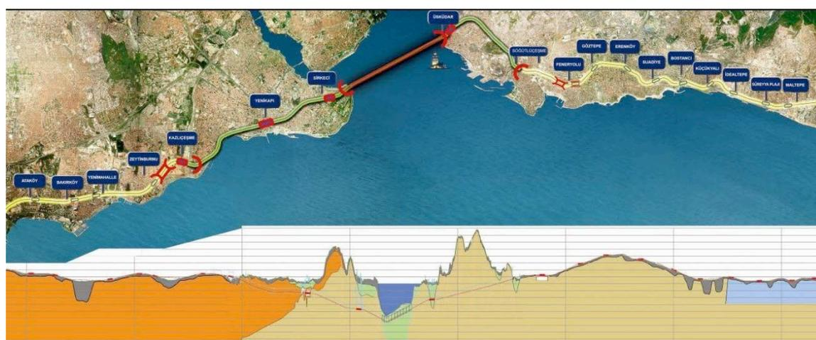
Fig. 1: The Marmaray Project Route Plan and Section (Altun&Baltaş, 2014: 30-31)
