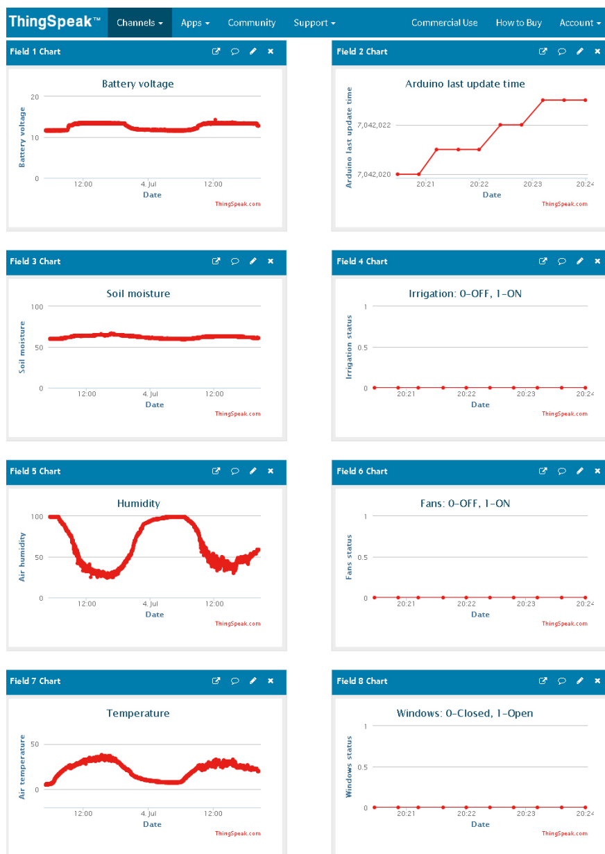
Figure 3 – Online server acting as data depository, as well as the communication link between the phone app and automated system. Source: https://thingspeak.com
