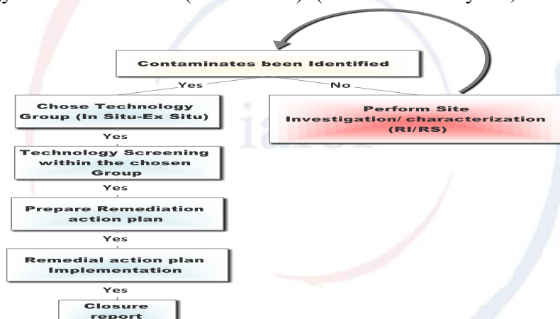
FIGURE 1 Contaminated Site Management and Technology Selection Process (CSM&TSP)
