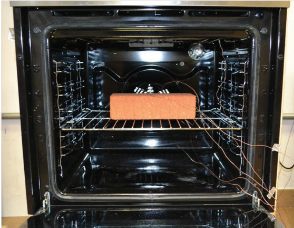
Figure 2. Position of the brick in the Normative Oven Energy Class Test: EN 50304.
