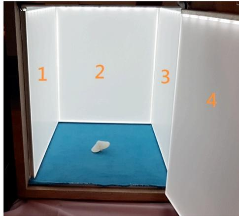
Figure 3: Four-sided LED lightening boarded recognition box
