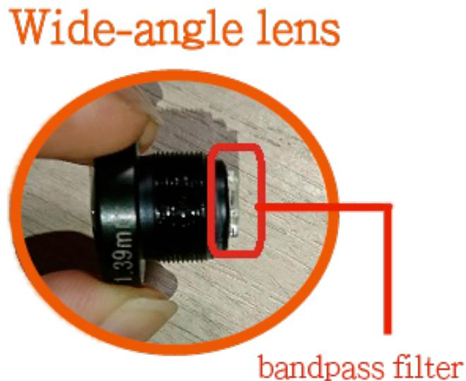
Figure 8: Wide-angle lens pasted with bandpass filter
