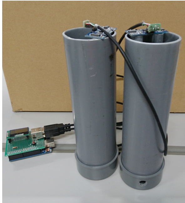
Fig. 2 Developed flow meter
