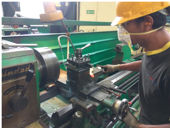
Figure 7: The use of coolant in machining process
