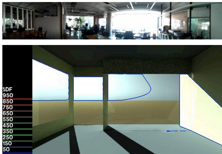
Figure 12: Above -Existing South side image of the Office, Below - Ecotect Simulation image | Source- Author
