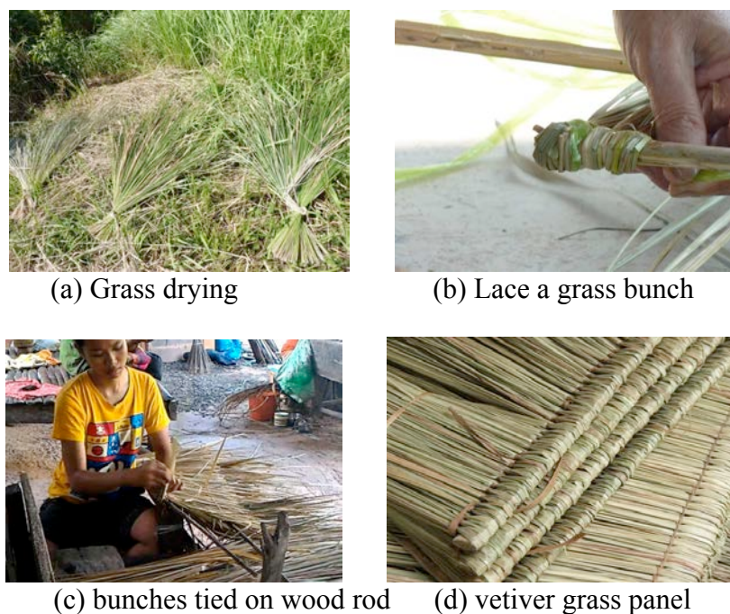
Figure 2. The process of vetiver roofing material manufacturing
