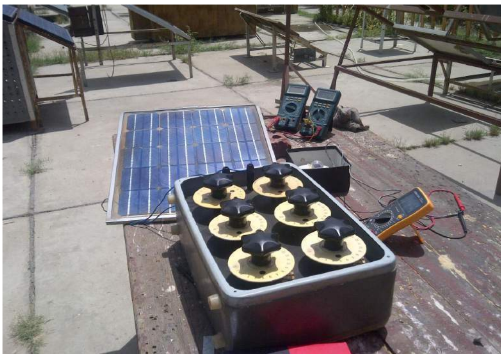
Fig. 4 Experimental PV measuring circuit.
