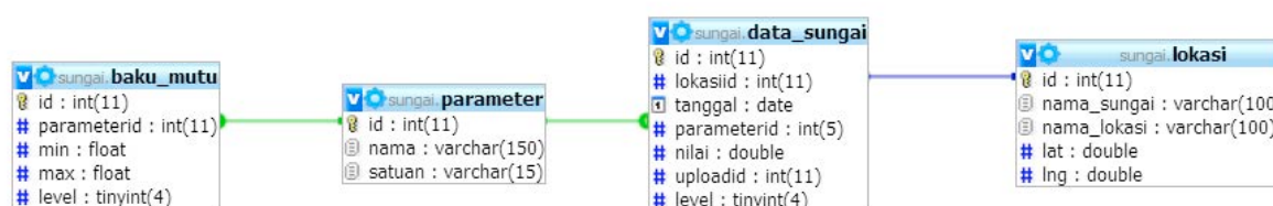
Fig. 4. Database schema of the river dashboard application
