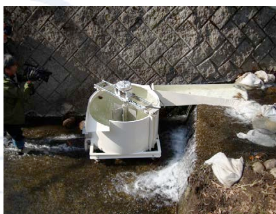
Fig. 3 On site test of a washbasin type hydropower generation (200 W max.)
