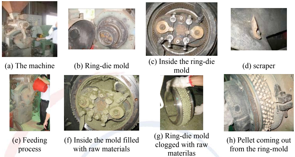
Figure 7 The appearance of ring-die molding machine (Yong-Ming YMHP-15)
