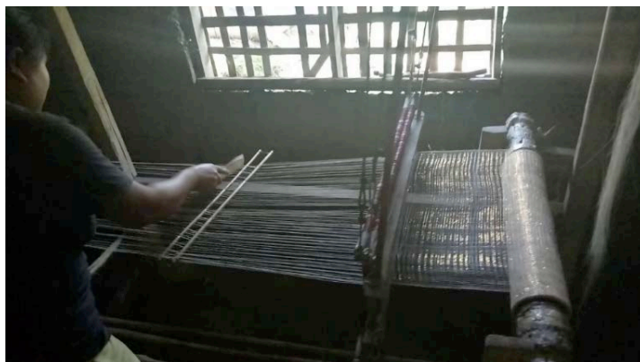
Figure 3. The Sinamay weaver while Combing the Abaca Strands in an Abulan .
