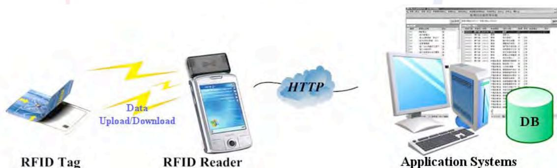
Figure 1. RFID Architecture
