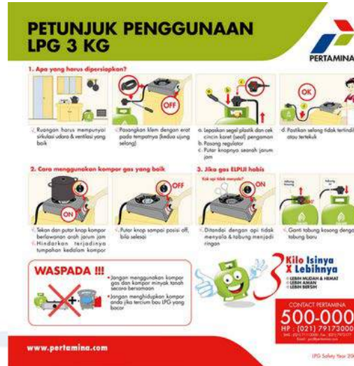
Example (2). The use of LPG cylinder. 1 Jun 2013. < http://iblogblog.blogspot.com/2010/07/cara-menggunakan-tabung-elpiji-3-kg.html >
