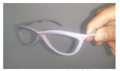
Figure 18: 3D printed frame.
