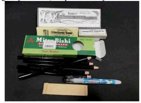
Figure 8: Plate drawing equipment that contain greasy ingredients
