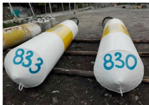
Figure 4. A cylindrical payao's buoy made of metal sheets painted and labelled at Purok Stella Maris, Tambler. Photo taken on February 19, 2017
