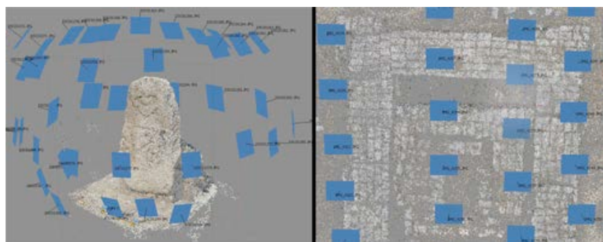
Figure 3: Terrestrial (left) and aerial acquisition procedure.
